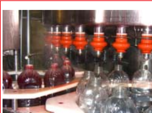
Bottles being filled with cranberry juice cocktail at the Seabrook, NJ plant.
